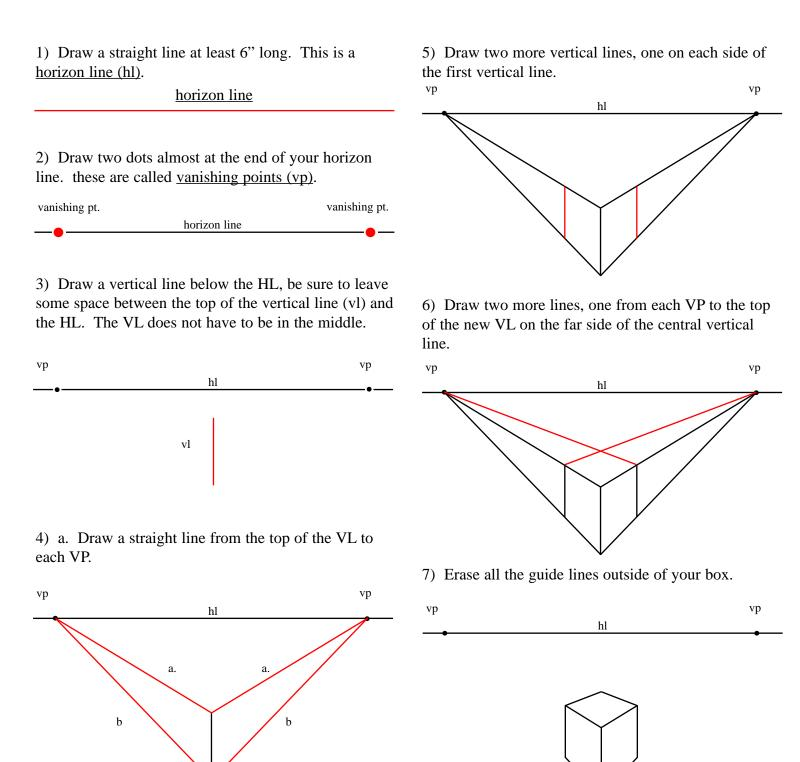
4) b. Draw a straight line from the bottom of the VL to each VP.
